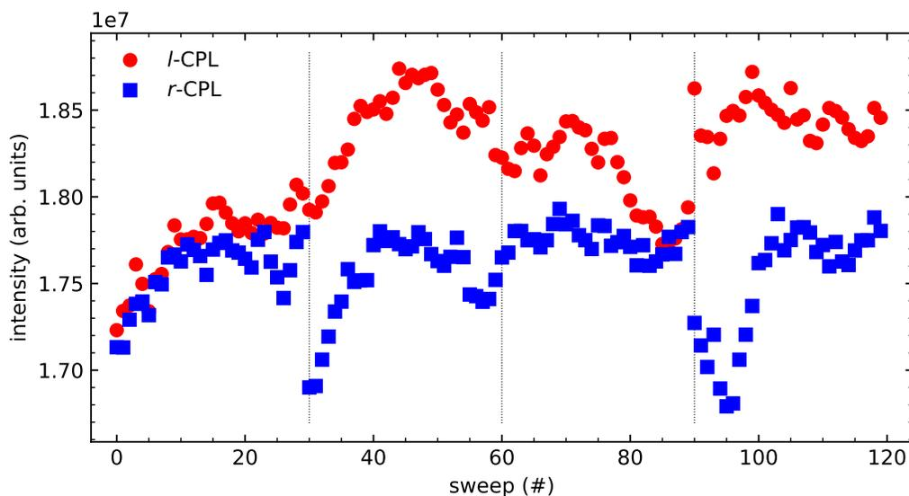
**Supplementary Fig. S2** Intensity fluctuations in series of photoelectron spectra from liquid (1S,4R)-fenchone. For each sweep, we show the summed intensity in units yielded by the acquisition software of the electron analyzer. The data shown for *l*-CPL correspond to the sweeps shown in Supplementary Fig. S1. The vertical dotted lines indicate a shift in helicity, performed after thirty sweeps. The acquisition started by recording sweeps 0-29 with *l*-CPL.
