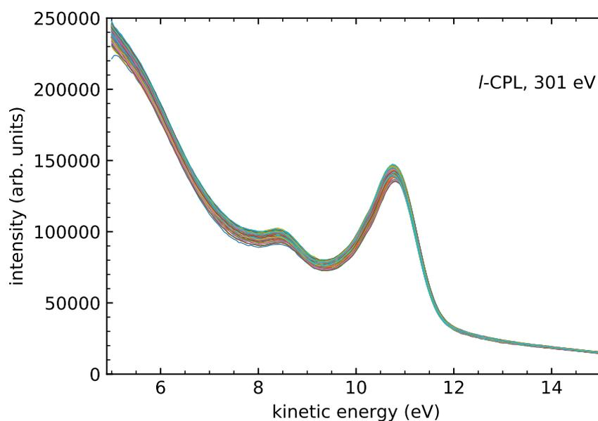
**Supplementary Fig. S1** Exemplary, single-sweep photoelectron spectra recorded from liquid (1S,4R)-fenchone, ionized with photons of 301 eV, see the sweep-averaged spectrum in Fig. 1 in the main article. Spectra were acquired in series of thirty sweeps each, with a change of photon helicity after each series. Here, traces from four series, recorded with *I*-CPL are shown. The spectra overlap due to the finite plot resolution.
