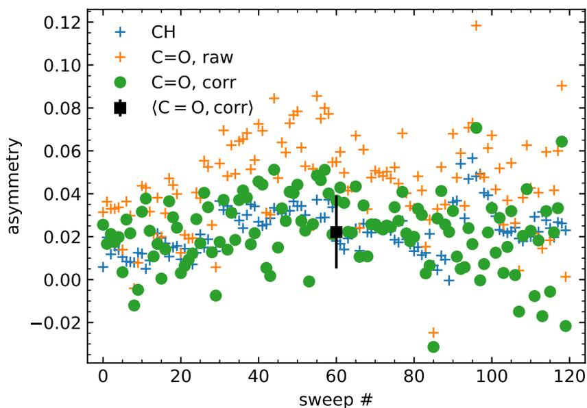
**Supplementary Fig. S5** Asymmetry  $A$  and corrected asymmetry  $A_{corr}$  calculated from the individual sweeps of the data set shown in Supplementary Fig. S1. The standard deviation of the set of corrected asymmetries is shown as an error bar to illustrate the data quality. The standard deviation of the mean is smaller than the symbol size. See the text for details.
