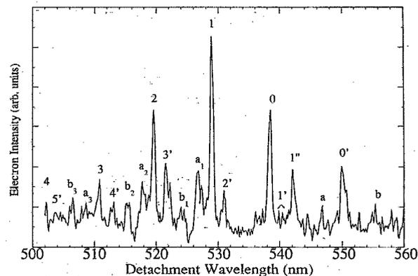
FIG. 2. Threshold photodetachment spectrum of  $\text{Si}_3^-$ .
