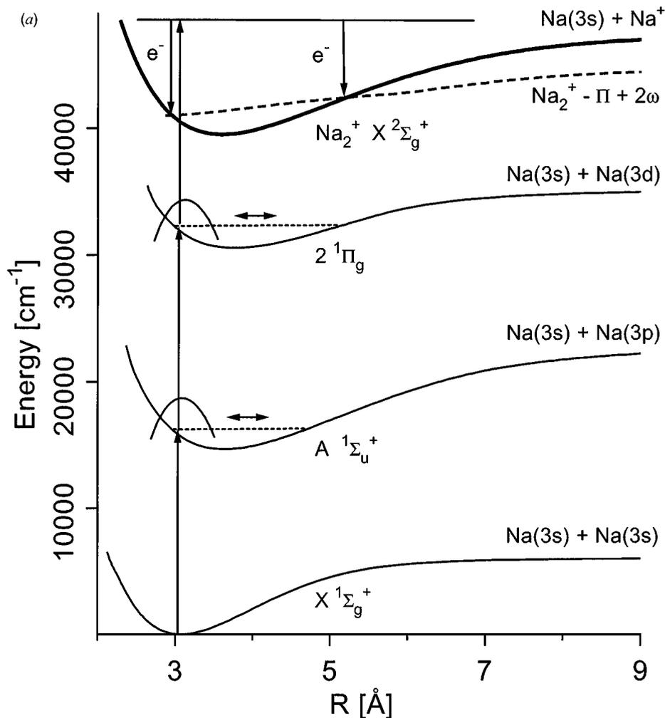
**Figure 2** Femtosecond PE spectroscopy of  $\text{Na}_2$ . Potential energy curves of  $\text{Na}_2$  and  $\text{Na}_2^+$  are shown in (a), while PE spectra showing coherent wavepacket motion on the excited  $\text{Na}_2$  states are shown in (b). Adapted from Reference (47).
