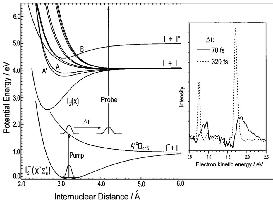
**Figure 1** Time-resolved photoelectron spectroscopy of  $I_2^-$ . Relevant potential energy curves for  $I_2^-$  and  $I_2$  are shown, along with PE spectra taken at pump-probe delay times of 70 and 320 fs.
